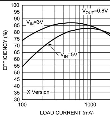
Figure 9. Efficiency vs Load, X Option
