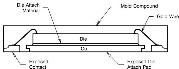
Figure 47. Internal Connection
