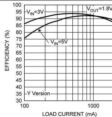
Figure 6. Efficiency vs Load, Y Option
