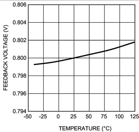
Figure 23.  $V_{FB}$  vs Temperature
