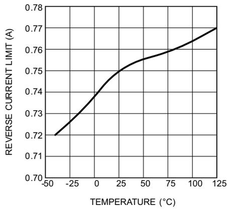
**Figure 25. Reverse Current Limit vs Temperature**
