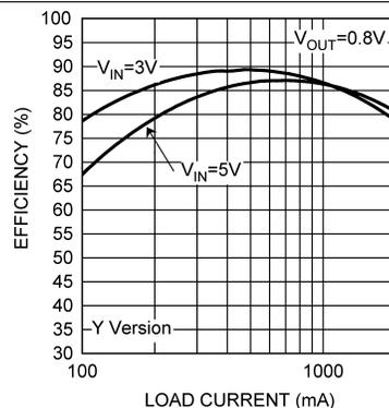
Figure 10. Efficiency vs Load, Y Option
