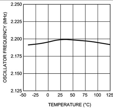
**Figure 15. Oscillator Frequency vs Temperature,, X Option**
