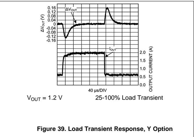
Figure 39. Load Transient Response, Y Option
