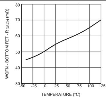
**Figure 18. R\_DS(on) Bottom Vs Temperature (WQFN-16 Package)**
