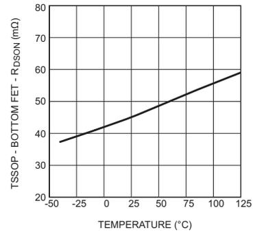
Figure 20.  $R_{DS(on)}$  Bottom vs Temperature (TSSOP-20 Package)
