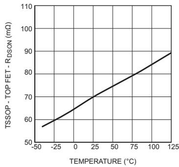
Figure 19.  $R_{DS(on)}$  Top vs Temperature (TSSOP-20 Package)
