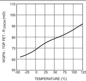
**Figure 17. R\_DS(on) Top Vs Temperature (WQFN-16 Package)**
