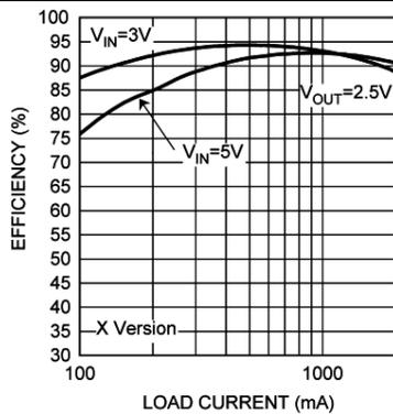
Figure 3. Efficiency vs Load, X Option
