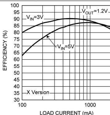
Figure 7. Efficiency vs Load, X Option
