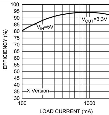
Figure 1. Efficiency vs Load, X Option
