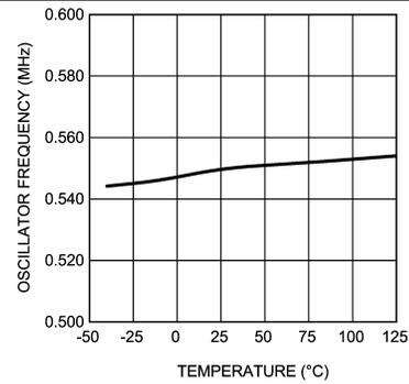
**Figure 16. Oscillator Frequency vs Temperature, Y Option**
