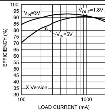
Figure 5. Efficiency vs Load, X Option
